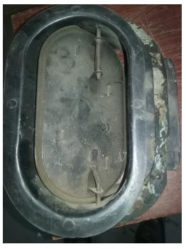
Another cold air entry is a missing grommet around speedo cable into the car. I
